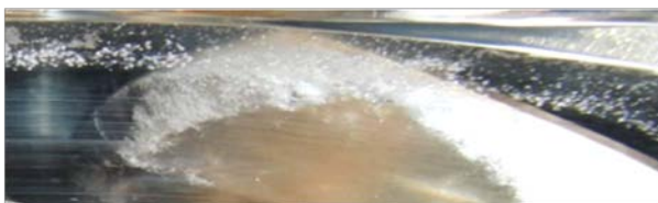
Fig. 4: Leading Edge Cavitation
